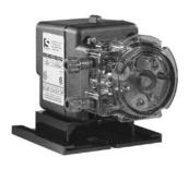
SWT's single head fixed output metering pump is built with two detachable components; the motor and the pump head. The fixed rate pump does not have an output adjustment. The output is determined by the rpm of the motor gears and the size of the pump tube. The motor's output shaft rotates at a fixed rpm which drives the roller assembly within the pump head.
